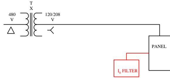
The Application of a Zero Sequence Harmonic Filter
