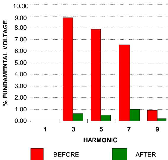
Harmonic Voltage Profiles for Non-Linear Loads with Harmonic Filtering Transformers
