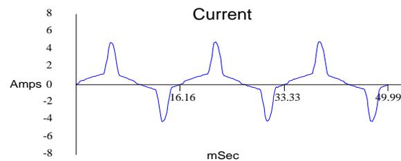
Current Waveform - Switch-Mode Power Supply
