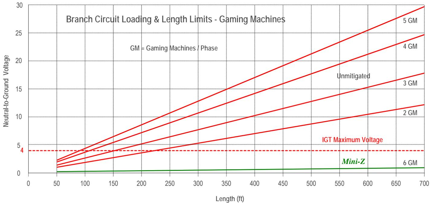
Neutral-to-Ground Voltage vs. Branch Circuit Loading and Length for Typical Non-Linear Electronic Gaming Machine Loads
