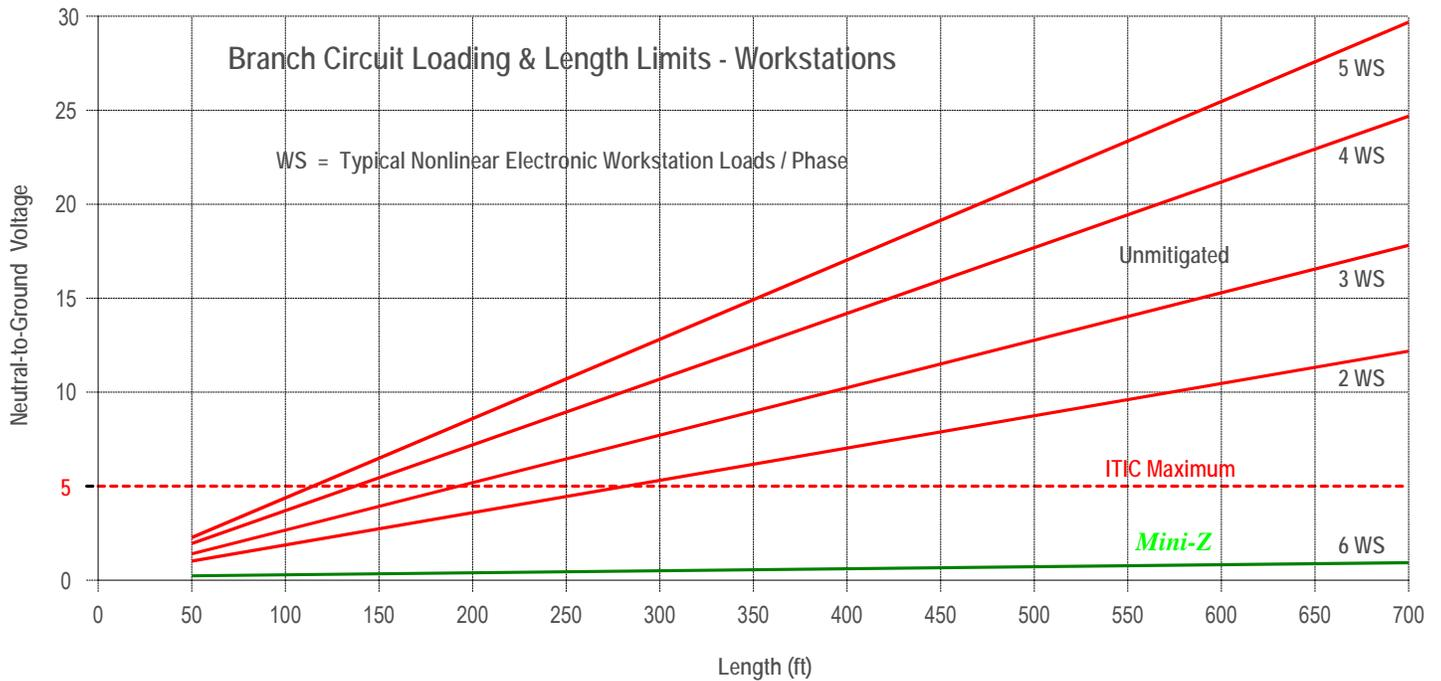
**Neutral-to-Ground Voltage vs. Branch Circuit Loading and Length for Typical Nonlinear Electronic Workstation Loads**
