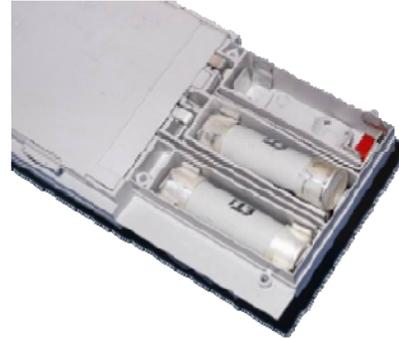
Step 4: The screw ejector lifts one end of the fuse, which may now be removed. Use of screw ejector mechanism avoids damaging the plastic tray.
