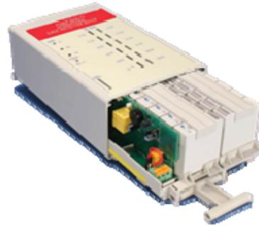
Step 1: Open the unit and remove the tray.
