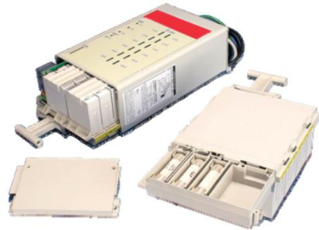
Step 4: Slide in the internal “tray”, and reattach the end mounting plate.
