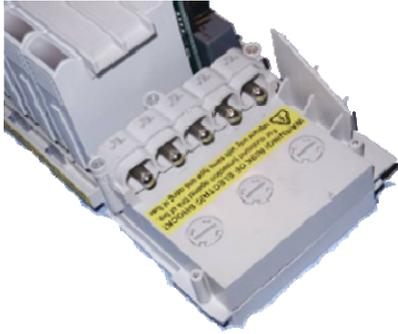
Step 3: Use a large flat blade screwdriver to turn the appropriate fuse ejector a quarter turn (90 degrees).
