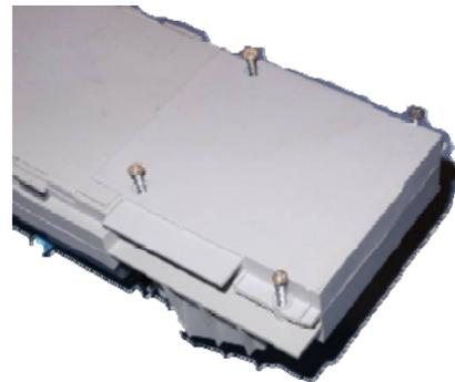
Step 2: Turn over, and remove the four screws holding the fuse cover in place. These screws are tight – use correct screwdriver size to avoid damaging screw head.
