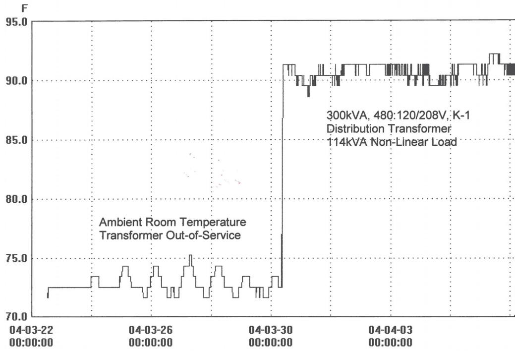
ELECTRICAL ROOM TEMPERATURES BEFORE TRANSFORMER REPLACEMENT
