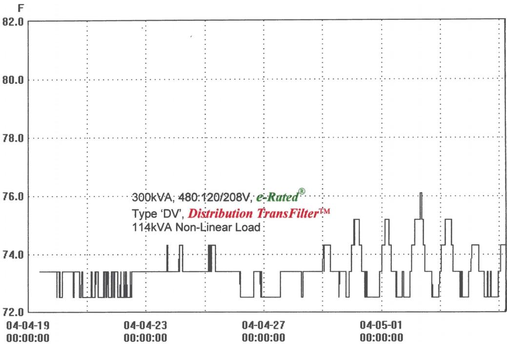
ELECTRICAL ROOM TEMPERATURES AFTER TRANSFORMER REPLACEMENT
